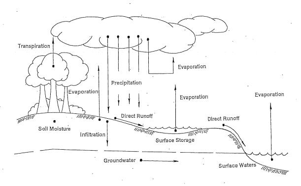
Figure 1 - Hydrologic Cycle
