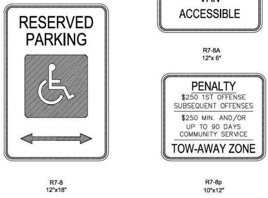
HANDICAPPED PARKING SIGNS
